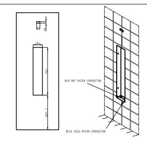
△ Linked the hot and cold water pipes, then tighten the screws (Attention: Filter washer must be installed to avoid dirt clogging), finally, paste up the tiles as the picture shows.
