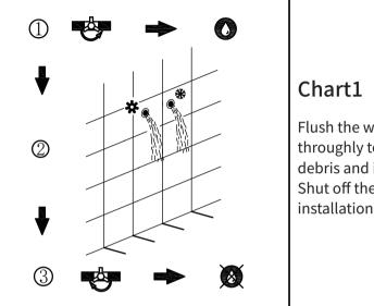
Flush the water supply lines throughly to drain debris and impurities.
