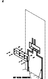
△ Put the concealed box into the slot on the wall, and fixed with the screws (no slipping, no loosening).
