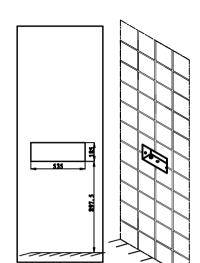
△Linked the hot and cold water pipes, then tighten the screws (Attention: Filter washer must be installed to avoid dirt clogging), finally, paste up the tiles as the picture shows.
