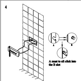
△Link the hot and cold water pipes accurately (please clean up the foreign body of connecting pipes before installation, and hang up the preassembled panel components in accordance with the picture shows (A must to all click into the B slot).
